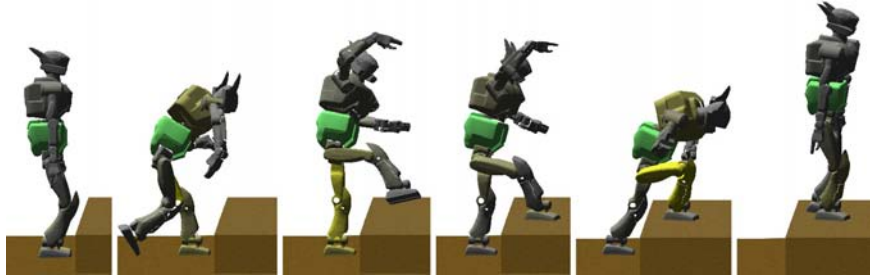
Fig. 4. Stair step planned entirely from scratch.
