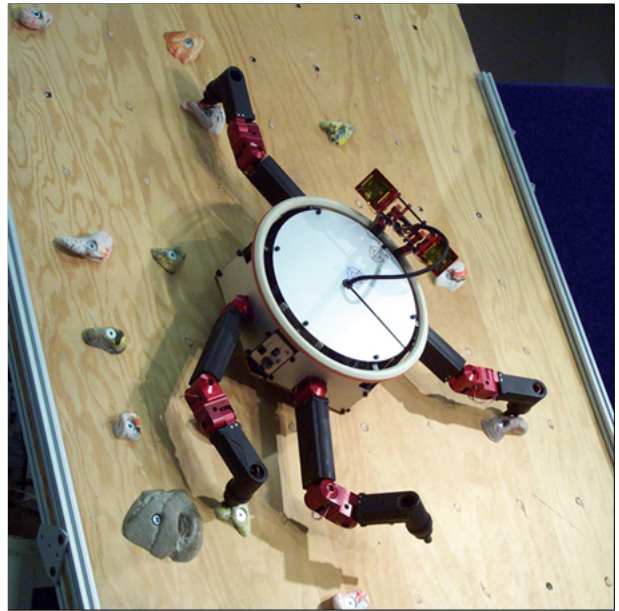
Fig. 1. The LEMUR IIB climbing robot [8].
